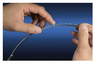
Pre-installed with connectors and fasteners, FlexRad® PMount™ snaps into any fixture assembly with the speed of a few button presses. Out of the package, PMount is completely ready to install and does not require special tools or jigs. The circuits can be shaped, curved, and trimmed to length at the time of installation. Just like all FlexRad products, PMount can be cut to length from reels that are up to hundreds of feet long.
